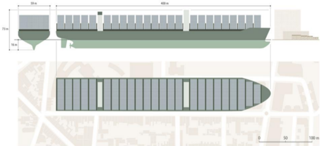
Esquema buque celular portacontenedores. (Fuente: International Transport Forum: The impact of Megaships, 2015)
