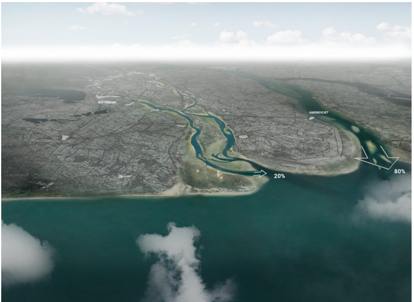
Aerial view of the mouths of the rivers Rhine and Meuse ca. 1850, before the construction of the Nieuwe Waterweg, seen from the west. The percentages indicate how the discharge of the rivers Rhine and Meuse is distributed to the different distributaries of the Rhine-Meuse delta. (© H+N+S Landscape Architects).
